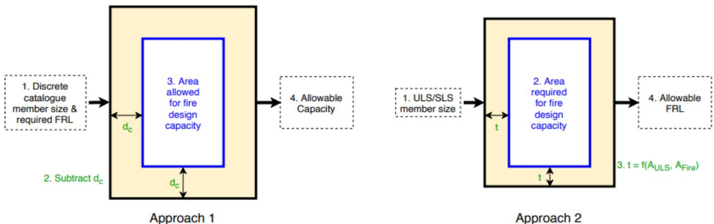
**Figure 1.** Schematic of the two design approaches to delivering a fire safe timber structure.
